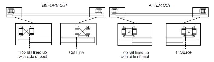
C) Join the railings together by sliding top and bottom rail into the post sleeves or into a loose wall mount.
