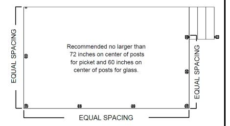
D) Once you have the posts placed into their positions, (approx. 2" from edge of the post base plate to edge of deck), pre-drill and loosely fasten the post to the deck with 1 fastener leaving 1/2" above the post base plate.
