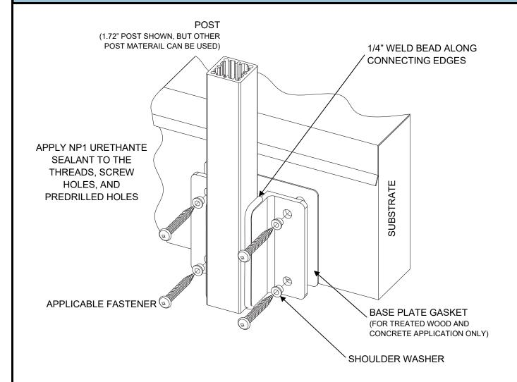
**SHOULDER WASHER:** These are put into the base plate mounting holes to prevent the stainless steel screw from marking the paint or coming in contact with the aluminum base plate, which could cause electrolysis. These can be purchased from the railing manufacturer.
